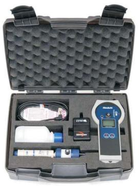
Soluble Salt Meter RPCT-07-001 for flat surfaces. 3ml fixed volume fluid dispenser 500 ml Container for deionized water Flexible plastic tubing to interconnect SSM and dispenser Universal AC adapter to charge the Li-ion battery of the SSM CD with SSM link software and manual USB connection cable 250 ml of 84 µS/cm validation fluid Syringe to inject validation fluid into the SSM
